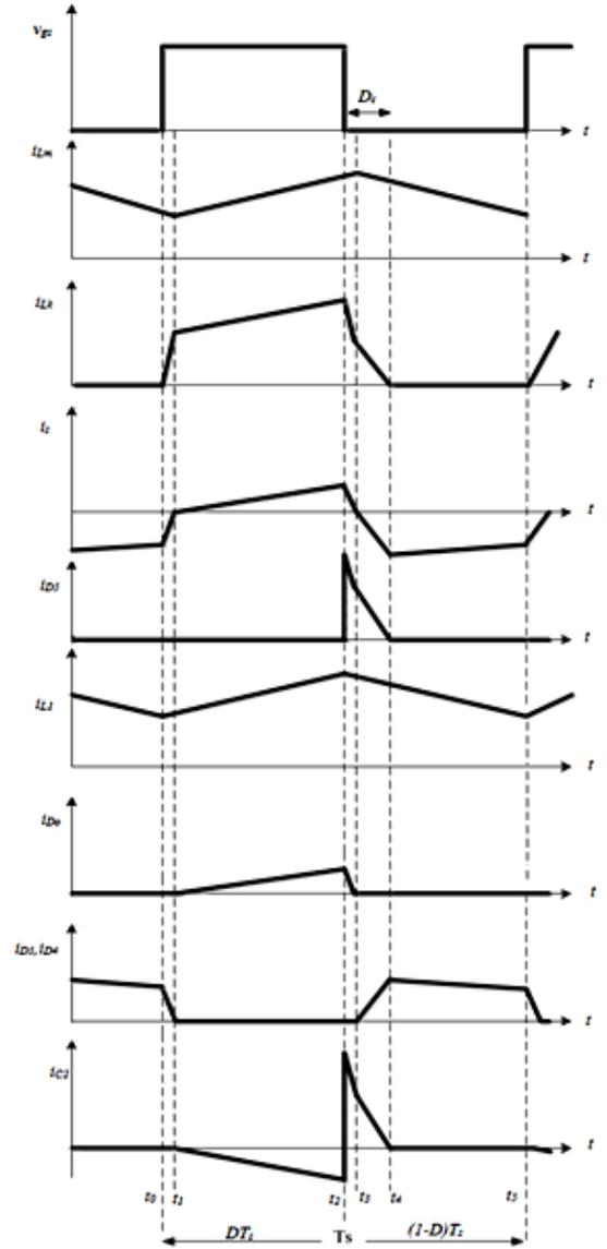
Fig. 2. Some typical waveforms of proposed converter at CCM operation
