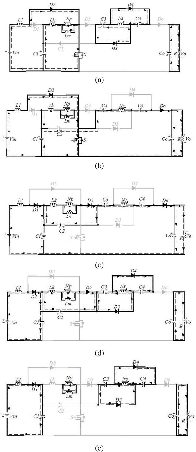
Fig. 3. Current flow paths of operating modes during on switching period at CCM operation. (a) Mode I. (b) Mode II. (c) Mode III. (d) Mode IV. (e) Mode V.
