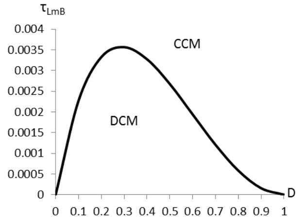
Fig. 9. Boundary condition of the proposed converter under  $n=2$
