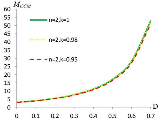
Fig. 6. Voltage gain versus duty cycle at CCM operation under  $n = 2$  and various  $k$ .
