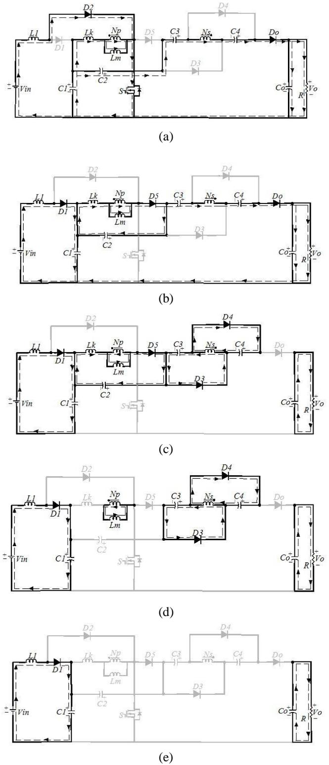
Fig. 5. Current flow paths of operating modes during on switching period at DCM operation. (a) Mode I. (b) Mode II. (c) Mode III. (d) Mode IV. (e) Mode V.
