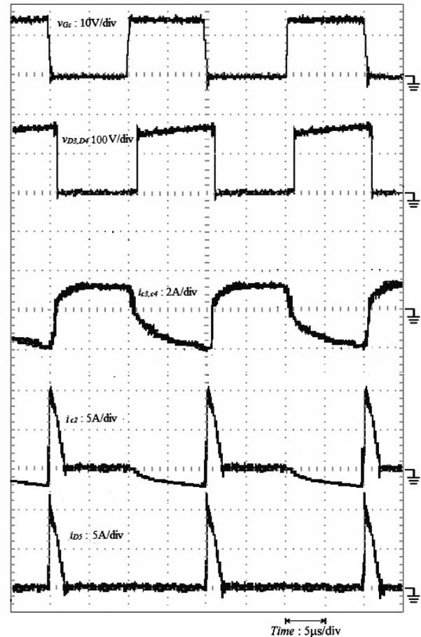
Fig. 12. Experimental result of some diodes and capacitor:  $V_{d3}$ ,  $V_{d4}$ ,  $V_{d5}$ ,  $I_{C3}$ ,  $I_{C4}$ ,  $I_{C2}$ , and  $I_{D5}$ , respectively.
