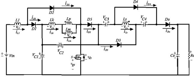
Fig. 1. Equivalent circuit configuration of the proposed converter
