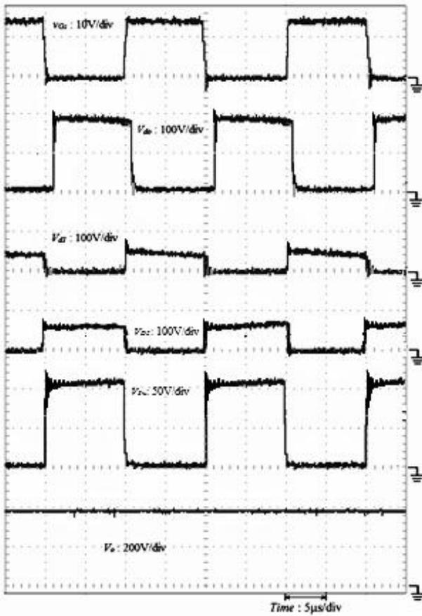
Fig. 10. Experimental result of the voltage stress on:  $V_{GS}$ ,  $V_{d1}$ ,  $V_{d2}$ ,  $V_{d3}$ , and  $V_o$ , respectively.
