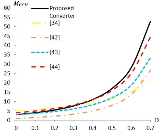
Fig. 7. Voltage gain versus duty ratio of the proposed converter and converters in [34],[42],[43] and [44] at CCM operation under  $n=2$  and  $k=1$
