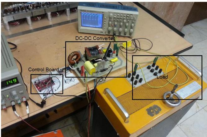
Fig. 15. Prototype of proposed converter
