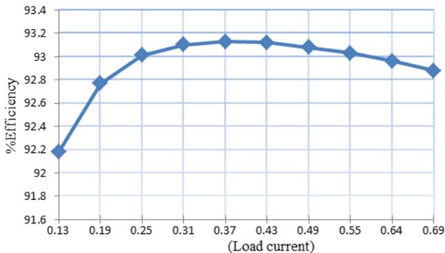
Fig. 14. Efficiency versus output current
