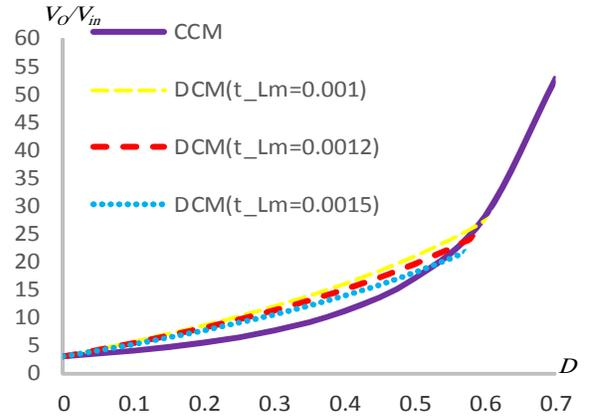
Fig. 8. Voltage gain versus duty ratio at DCM operation under various  $\tau_{Lm}$  value and CCM operation under  $n=2$  and  $k=1$
