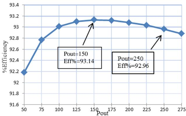
Fig. 13. Efficiency versus output power
