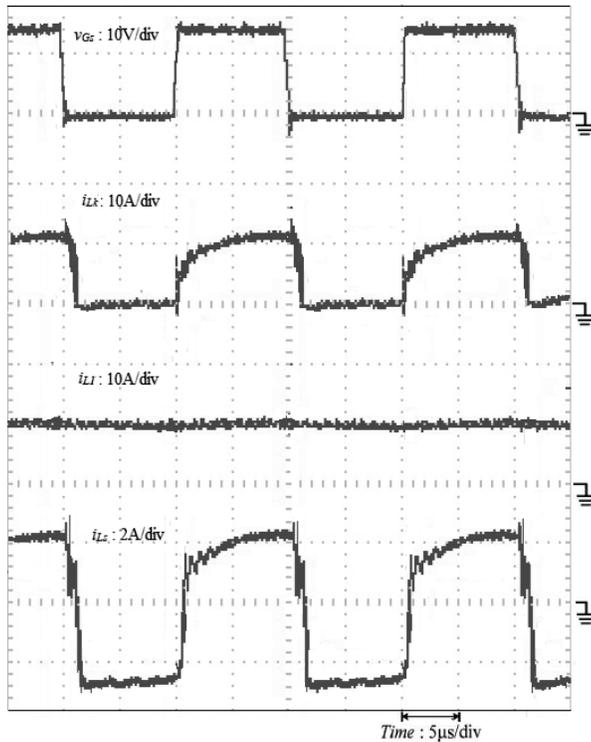
Fig. 11. Experimental result of the current waveform of  $i_{Lk}$ ,  $i_{Ll}$  and  $i_s$ , respectively.
