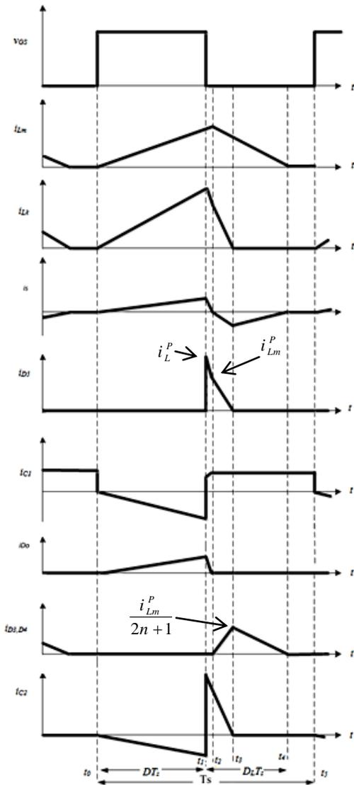
Fig. 4. Some typical waveforms of proposed converter at DCM operation
